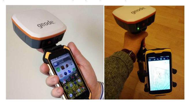
Optional accessories include lightweight, telescopic monopod and clamp (pictured right, not extended) and backpack to hold pole and Geode.
